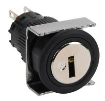
Fuji Electric selector switch, IP65, 19mm, 3-position, spring return to center from left, maintained right, key removable center and right position, DPDT contact(s), plastic base, plastic bezel, Operator: silver, key, 22mm, round, metal.
