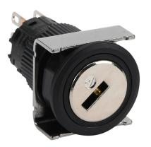
Fuji Electric selector switch, IP65, 19mm, 3-position, spring return to center from left, maintained right, key removable right position, DPDT contact(s), plastic base, plastic bezel, Operator: silver, key, 22mm, round, metal.
