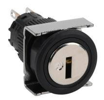
Fuji Electric selector switch, IP65, 19mm, 3-position, maintained, key removable center position, DPDT contact(s), plastic base, plastic bezel, Operator: silver, key, 22mm, round, metal.
