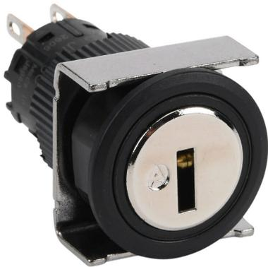
Fuji Electric selector switch, IP65, 19mm, 3-position, maintained, key removable left, right and center position, DPDT contact(s), plastic base, plastic bezel, Operator: silver, key, 22mm, round, metal.
