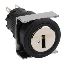
Fuji Electric selector switch, IP65, 19mm, 3-position, maintained, key removable left, right and center position, DPDT contact(s), plastic base, plastic bezel, Operator: silver, key, 22mm, round, metal.
