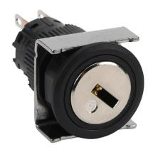
Fuji Electric selector switch, IP65, 19mm, 2-position, maintained, key removable left and right position, DPDT contact(s), plastic base, plastic bezel, Operator: silver, key, 22mm, round, metal.
