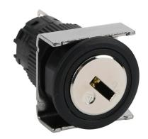
Fuji Electric selector switch, IP65, 19mm, 2-position, maintained, key removable left and right position, SPDT contact(s), plastic base, plastic bezel, Operator: silver, key, 22mm, round, metal.
