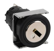
Fuji Electric selector switch, IP65, 19mm, 2-position, maintained, key removable left position, SPDT contact(s), plastic base, plastic bezel, Operator: silver, key, 22mm, round, metal.
