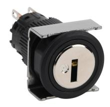
Fuji Electric selector switch, IP65, 19mm, 3-position, spring return to center from right or left, key removable center position, DPDT contact(s), plastic base, plastic bezel, Operator: silver, key, 22mm, round, metal.
