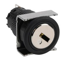
Fuji Electric selector switch, IP65, 19mm, 2-position, spring return from right, key removable left position, SPDT contact(s), plastic base, plastic bezel, Operator: silver, key, 22mm, round, metal.
