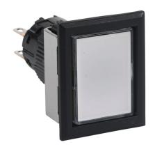
Fuji Electric pushbutton, IP65, 16mm, push ON - push OFF, DPDT contact(s), plastic base, plastic bezel, black, Operator: white, flush, 28mm, rectangular, plastic.
