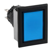
Fuji Electric pushbutton, IP65, 16mm, push ON - push OFF, DPDT contact(s), plastic base, plastic bezel, black, Operator: blue, flush, 28mm, rectangular, plastic.
