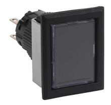
Fuji Electric pushbutton, IP65, 16mm, push ON - push OFF, DPDT contact(s), plastic base, plastic bezel, black, Operator: black, flush, 28mm, rectangular, plastic.
