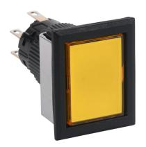
Fuji Electric pushbutton, IP65, 16mm, push ON - push OFF, LED illuminated, DPDT contact(s), plastic base, plastic bezel, black, Operator: yellow, flush, 28mm, rectangular, plastic, 24 VAC/VDC, full voltage.
