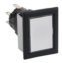
Fuji Electric pushbutton, IP65, 16mm, push ON - push OFF, LED illuminated, DPDT contact(s), plastic base, plastic bezel, black, Operator: white, flush, 28mm, rectangular, plastic, 24 VAC/VDC, full voltage.
