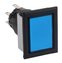
Fuji Electric pushbutton, IP65, 16mm, push ON - push OFF, LED illuminated, DPDT contact(s), plastic base, plastic bezel, black, Operator: blue, flush, 28mm, rectangular, plastic, 24 VAC/VDC, full voltage.
