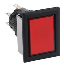
Fuji Electric pushbutton, IP65, 16mm, push ON - push OFF, LED illuminated, DPDT contact(s), plastic base, plastic bezel, black, Operator: red, flush, 28mm, rectangular, plastic, 24 VAC/VDC, full voltage.
