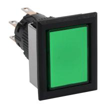
Fuji Electric pushbutton, IP65, 16mm, push ON - push OFF, LED illuminated, DPDT contact(s), plastic base, plastic bezel, black, Operator: green, flush, 28mm, rectangular, plastic, 24 VAC/VDC, full voltage.
