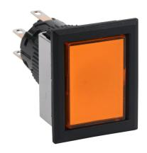
Fuji Electric pushbutton, IP65, 16mm, push ON - push OFF, LED illuminated, DPDT contact(s), plastic base, plastic bezel, black, Operator: orange, flush, 28mm, rectangular, plastic, 24 VAC/VDC, full voltage.
