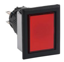
Fuji Electric pushbutton, IP65, 16mm, momentary, DPDT contact(s), plastic base, plastic bezel, black, Operator: red, flush, 28mm, rectangular, plastic.
