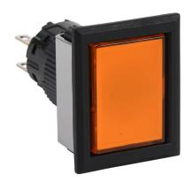
Fuji Electric pushbutton, IP65, 16mm, momentary, DPDT contact(s), plastic base, plastic bezel, black, Operator: orange, flush, 28mm, rectangular, plastic.
