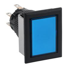
Fuji Electric pushbutton, IP65, 16mm, momentary, LED illuminated, DPDT contact(s), plastic base, plastic bezel, black, Operator: blue, flush, 28mm, rectangular, plastic, 24 VAC/VDC, full voltage.
