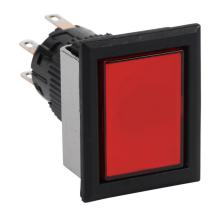
Fuji Electric pushbutton, IP65, 16mm, momentary, LED illuminated, DPDT contact(s), plastic base, plastic bezel, black, Operator: red, flush, 28mm, rectangular, plastic, 24 VAC/VDC, full voltage.
