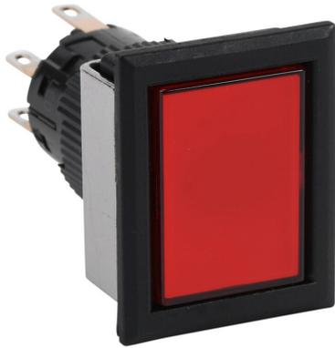
Fuji Electric pushbutton, IP65, 16mm, momentary, LED illuminated, DPDT contact(s), plastic base, plastic bezel, black, Operator: red, flush, 28mm, rectangular, plastic, 24 VAC/VDC, full voltage.
