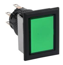
Fuji Electric pushbutton, IP65, 16mm, momentary, LED illuminated, DPDT contact(s), plastic base, plastic bezel, black, Operator: green, flush, 28mm, rectangular, plastic, 24 VAC/VDC, full voltage.
