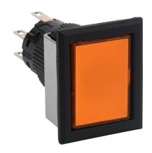
Fuji Electric pushbutton, IP65, 16mm, momentary, LED illuminated, DPDT contact(s), plastic base, plastic bezel, black, Operator: orange, flush, 28mm, rectangular, plastic, 24 VAC/VDC, full voltage.
