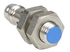
Micro Detectors inductive proximity sensor, tubular, 8mm diameter x 29.4mm body, stainless steel housing, PNP, N.C. output, 2mm sensing distance, flush, 7 kHz switching frequency, IP67, 3-pin M8 quick-disconnect.
