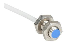
Micro Detectors inductive proximity sensor, tubular, 8mm diameter x 20.3mm body, stainless steel housing, PNP, N.C. output, 2mm sensing distance, flush, 7 kHz switching frequency, IP67, pigtail.
