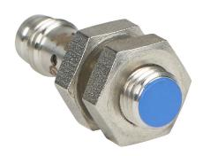
Micro Detectors inductive proximity sensor, tubular, 8mm diameter x 29.4mm body, stainless steel housing, PNP, N.C. output, 1.5mm sensing distance, flush, 7 kHz switching frequency, IP67, 3-pin M8 quick-disconnect.
