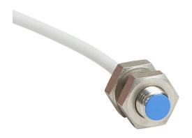
Micro Detectors inductive proximity sensor, tubular, 8mm diameter x 20.3mm body, stainless steel housing, PNP, N.C. output, 1.5mm sensing distance, flush, 7 kHz switching frequency, IP67, pigtail.
