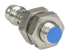
Micro Detectors inductive proximity sensor, tubular, 8mm diameter x 29.4mm body, stainless steel housing, NPN, N.C. output, 2mm sensing distance, flush, 7 kHz switching frequency, IP67, 3-pin M8 quick-disconnect.
