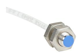
Micro Detectors inductive proximity sensor, tubular, 8mm diameter x 20.3mm body, stainless steel housing, NPN, N.C. output, 2mm sensing distance, flush, 7 kHz switching frequency, IP67, pigtail.
