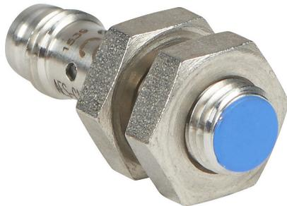
Micro Detectors inductive proximity sensor, tubular, 8mm diameter x 29.4mm body, stainless steel housing, NPN, N.C. output, 1.5mm sensing distance, flush, 7 kHz switching frequency, IP67, 3-pin M8 quick-disconnect.
