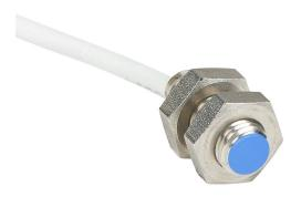
Micro Detectors inductive proximity sensor, tubular, 8mm diameter x 20.3mm body, stainless steel housing, NPN, N.C. output, 1.5mm sensing distance, flush, 7 kHz switching frequency, IP67, pigtail.
