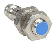
Micro Detectors inductive proximity sensor, tubular, 8mm diameter x 29.4mm body, stainless steel housing, PNP, N.O. output, 2mm sensing distance, flush, 7 kHz switching frequency, IP67, 3-pin M8 quick-disconnect.
