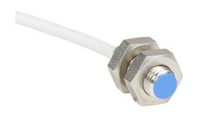
Micro Detectors inductive proximity sensor, tubular, 8mm diameter x 20.3mm body, stainless steel housing, PNP, N.O. output, 2mm sensing distance, flush, 7 kHz switching frequency, IP67, pigtail.
