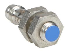
Micro Detectors inductive proximity sensor, tubular, 8mm diameter x 29.4mm body, stainless steel housing, PNP, N.O. output, 1.5mm sensing distance, flush, 7 kHz switching frequency, IP67, 3-pin M8 quick-disconnect.
