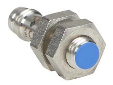
Micro Detectors inductive proximity sensor, tubular, 8mm diameter x 29.4mm body, stainless steel housing, PNP, N.O. output, 1.5mm sensing distance, flush, 7 kHz switching frequency, IP67, 3-pin M8 quick-disconnect.
