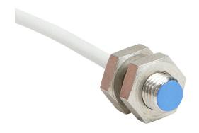
Micro Detectors inductive proximity sensor, tubular, 8mm diameter x 20.3mm body, stainless steel housing, PNP, N.O. output, 1.5mm sensing distance, flush, 7 kHz switching frequency, IP67, pigtail.
