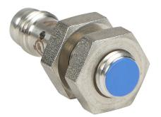
Micro Detectors inductive proximity sensor, tubular, 8mm diameter x 29.4mm body, stainless steel housing, NPN, N.O. output, 2mm sensing distance, flush, 7 kHz switching frequency, IP67, 3-pin M8 quick-disconnect.
