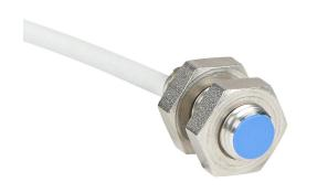
Micro Detectors inductive proximity sensor, tubular, 8mm diameter x 20.3mm body, stainless steel housing, NPN, N.O. output, 2mm sensing distance, flush, 7 kHz switching frequency, IP67, pigtail.
