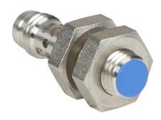
Micro Detectors inductive proximity sensor, tubular, 8mm diameter x 29.4mm body, stainless steel housing, NPN, N.O. output, 1.5mm sensing distance, flush, 7 kHz switching frequency, IP67, 3-pin M8 quick-disconnect.
