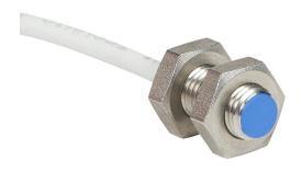
Micro Detectors inductive proximity sensor, tubular, 8mm diameter x 20.3mm body, stainless steel housing, NPN, N.O. output, 1.5mm sensing distance, flush, 7 kHz switching frequency, IP67, pigtail.
