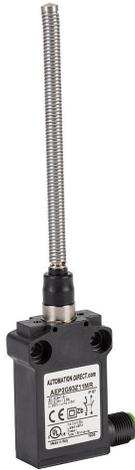
AutomationDirect compact limit switch, 360 degree stainless steel spring, (1) N.O./(1) N.C. contact(s), snap action, 25mm hole spacing, plastic, (1) 5-pin M12 quick-disconnect, right exit.
