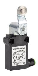
AutomationDirect compact limit switch, side rotary lever with 14mm metal roller, (1) N.O./(1) N.C. contact(s), snap action, 25mm hole spacing, plastic, (1) 5-pin M12 quick-disconnect, right exit.
