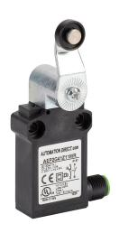
AutomationDirect compact limit switch, side rotary lever with 14mm nylon roller, (1) N.O./(1) N.C. contact(s), snap action, 25mm hole spacing, plastic, (1) 5-pin M12 quick-disconnect, right exit.
