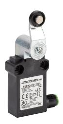
AutomationDirect compact limit switch, side rotary lever with 14mm nylon roller, (1) N.O./(1) N.C. contact(s), snap action, 25mm hole spacing, plastic, 5-pin M12 quick-disconnect, right exit.
