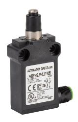
AutomationDirect compact limit switch, metal plunger with dust cap, (1) N.O./(1) N.C. contact(s), snap action, 25mm hole spacing, plastic, (1) 5-pin M12 quick-disconnect, right exit.
