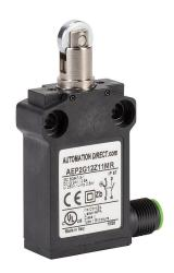
AutomationDirect compact limit switch, metal plunger with metal roller, (1) N.O./(1) N.C. contact(s), snap action, 25mm hole spacing, plastic, (1) 5-pin M12 quick-disconnect, right exit.
