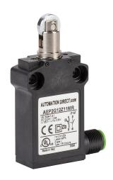
AutomationDirect compact limit switch, metal plunger with metal roller, (1) N.O./(1) N.C. contact(s), snap action, 25mm hole spacing, plastic, 5-pin M12 quick-disconnect, right exit.
