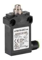
AutomationDirect compact limit switch, metal plunger, (1) N.O./ (1) N.C. contact(s), snap action, 25mm hole spacing, plastic, (1) 5-pin M12 quick-disconnect, right exit.
