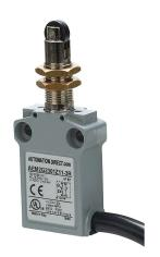
AutomationDirect compact limit switch, metal plunger with nylon roller with fixing nuts, (1) N.O./(1) N.C. contact(s), snap action, 25mm hole spacing, zinc alloy, pigtail, 9.8ft/3m cable length, right exit.
