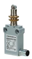
AutomationDirect compact limit switch, metal plunger with metal roller and fixing nuts, (1) N.O./(1) N.C. contact(s), snap action, 25mm hole spacing, zinc alloy, (1) 5-pin M12 quick-disconnect, right exit.
