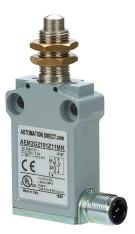
AutomationDirect compact limit switch, metal plunger with fixing nuts, (1) N.O./(1) N.C. contact(s), snap action, 25mm hole spacing, zinc alloy, (1) 5-pin M12 quick-disconnect, right exit.
