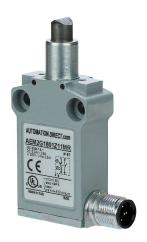
AutomationDirect compact limit switch, metal plunger with bevel cut, (1) N.O./(1) N.C. contact(s), snap action, 25mm hole spacing, zinc alloy, 5-pin M12 quick-disconnect, right exit.
